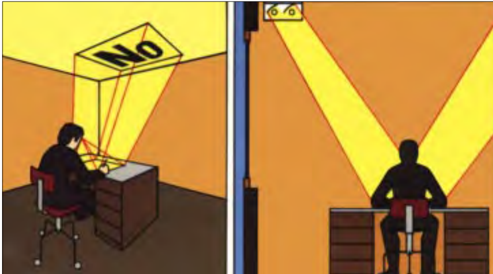
Fig. 9.8 Distribution of luminous intensity of a luminaire, which minimizes reflected glare
