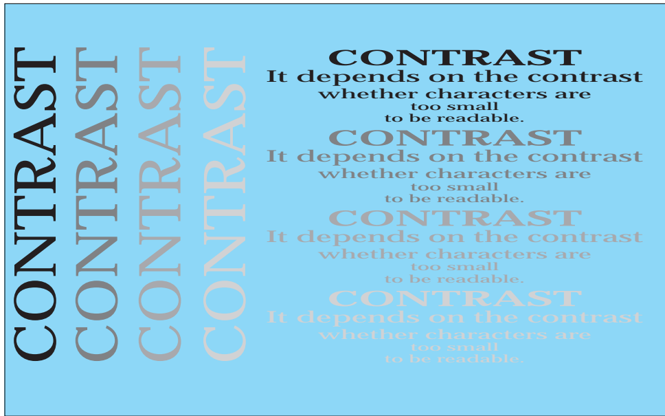
Fig. 9.10 Changes in the readability of a text under lighting arrangements with different contrast rendering factors. (Note: The effect is easily to demonstrate with a glossy magazine under direct lighting.)
