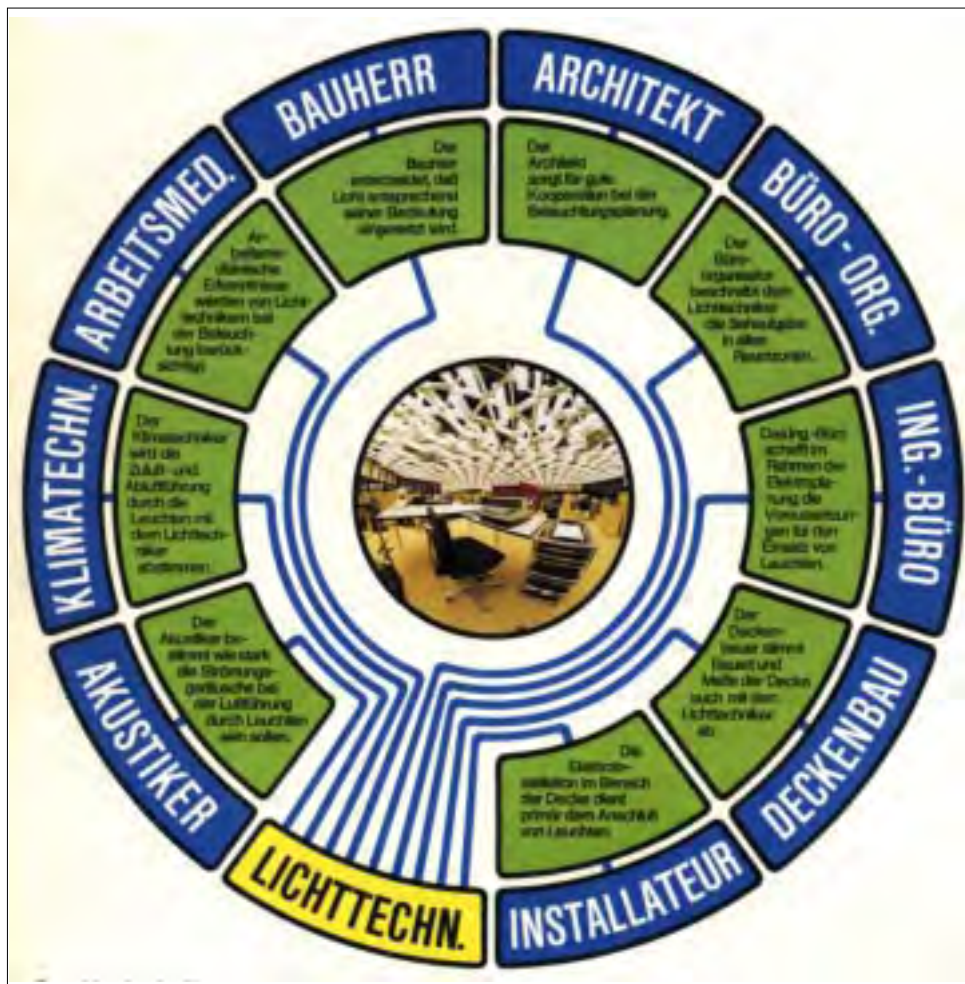
Fig 10.1 Idealized representation of the cooperation between persons and groups involved in planning on the one hand and the lighting engineer (bottom, left) on the other. (Source: FGL) (clockwise from lighting engineer: Consultants: acoustics, air-conditioning, occupational medicine; client, architect, office organizer; engineers: electrical engineer, ceiling, electrical installation)
